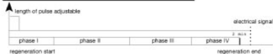
Example 5 stage valve with external signal
